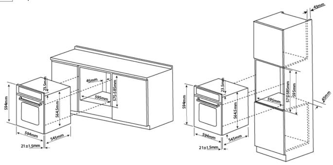
NOTE: Dimensions provided above for the cut-out are for a face mount only!
