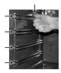
To remove the side support racks, push down on the wire below the locking pin, pull away from the oven wall until you can release the bottom of the support from the holes in the oven wall. To replace, reverse this procedure.
